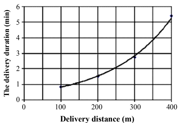
Fig. 4: The dependence of ore delivery duration from the distance
