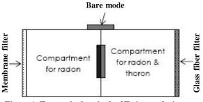
Figure 1: Entrenched outlook of Twin cup dosimeter
