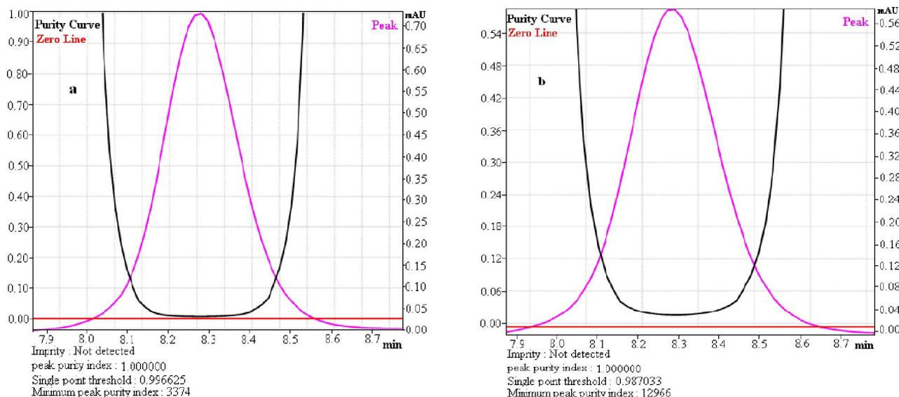
**Figure 7 : Representative peak purity curve of itaconic acid in mobile phase (a) and in hydrogel matrix (b) each of the peak has a positive value of minimum peak purity index confirming the purity of the peaks and specificity**
