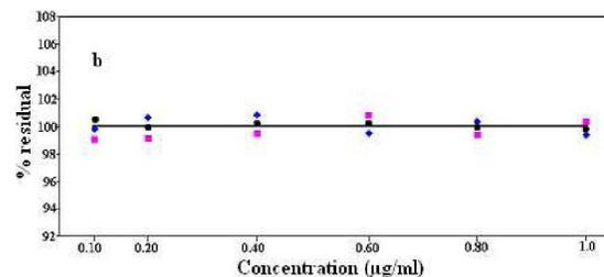
**Figure 3 :** Linearity curve of itaconic acid (a), Residual plot: Assessment of linearity (for a better view only three readings are shown for each calibration point)
