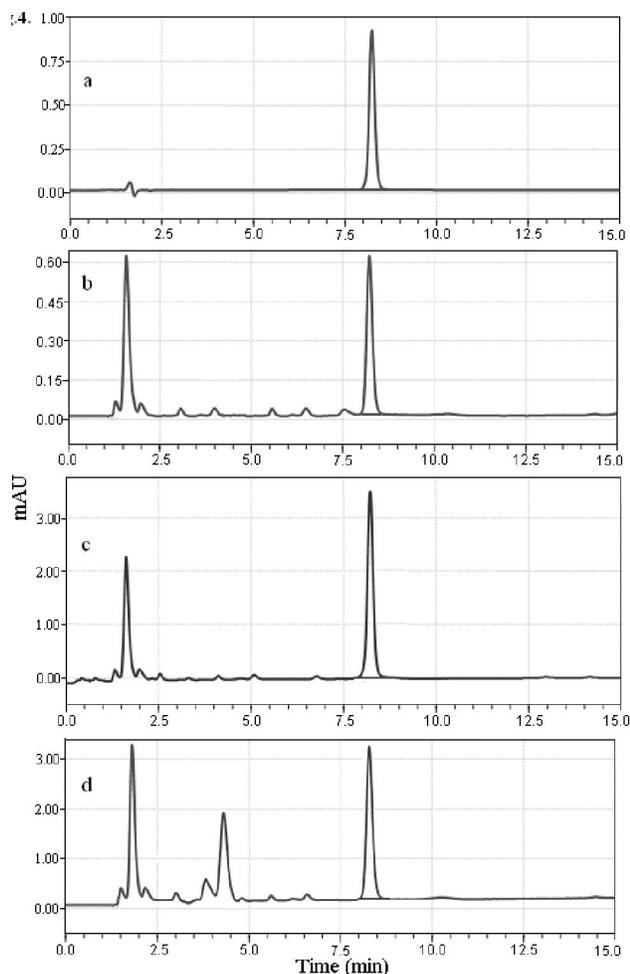
**Figure 4 :** Representative HPLC chromatograms of standard itaconic acid (0.2mg/ml) (a), fortified in PAM gel (4 µg/ml) (b), residual itaconic acid detected in P (AM-co-IA) (c) and in collagen-g-p (AM-co-IA) hydrogel (d)
