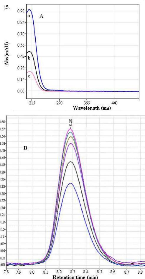
**Figure 5 :** (A) Absorption spectrum of itaconic acid (0.2mg/ml) in the mobile phase (measured at height h (a), h/2 (b) and h/4 (c) respectively). No changes in spectral pattern was observed. (B) Itaconic acid fortified (4.0mg/ml) was detected at the wavelengths of 210, 200, 212, 215, 220 and 222 nm simultaneously
