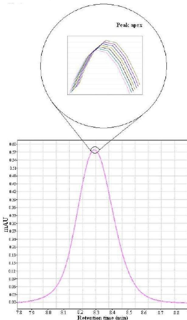
**Figure 6 :** Overlay of signals of itaconic acid fortified (4.0mg/ml) at wavelengths 210, 200, 212, 215, 220, and 222 nm after normalized to equal areas
