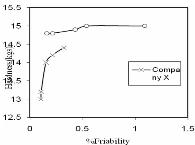
**Fig. 2: % Friability vs hardness (Ferrous fumarate)**
