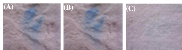
Figure 8 : Washing performance of protease from B. subtilis in the presence of detergent (Wheel). (A): Cloth stained with ink (B): Ink-stained cloth washed with detergent only (C): Ink-stained cloth washed with detergent and enzyme.
