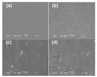
Figure 2 : SEM micrographs of film surfaces of (a) chitosan and chitosan nanocomposite films prepared using chitosan/ MPEG-*b*-PDLL ratios of (b) 90/10, (c) 80/20 and (d) 70/30 (w/w). All bars = 1  $\mu$ m.
