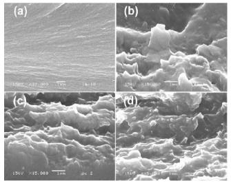
Figure 3 : SEM micrographs of film cross-sections of (a) chitosan and chitosan nanocomposite films prepared using chitosan/MPEG-*b*-PDLL ratios of (b) 90/10, (c) 80/20 and (d) 70/30 (w/w). All bars = 1  $\mu$ m.
