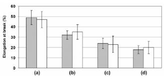
Figure 6 : Elongations at break in dry (■) and hydrated (□) states of (a) chitosan film and chitosan nanocomposite films prepared using chitosan/MPEG-*b*-PDLL ratios of (b) 90/10, (c) 80/20 and (d)70/30 (w/w).
