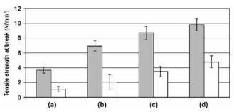
Figure 5 : Tensile strengths at break in dry ( $\blacksquare$ ) and hydrated ( $\Box$ ) states of (a) chitosan film and chitosan nanocomposite films prepared using chitosan/MPEG-*b*-PDLL ratios of (b) 90/10, (c) 80/20 and (d)70/30 (w/w).
