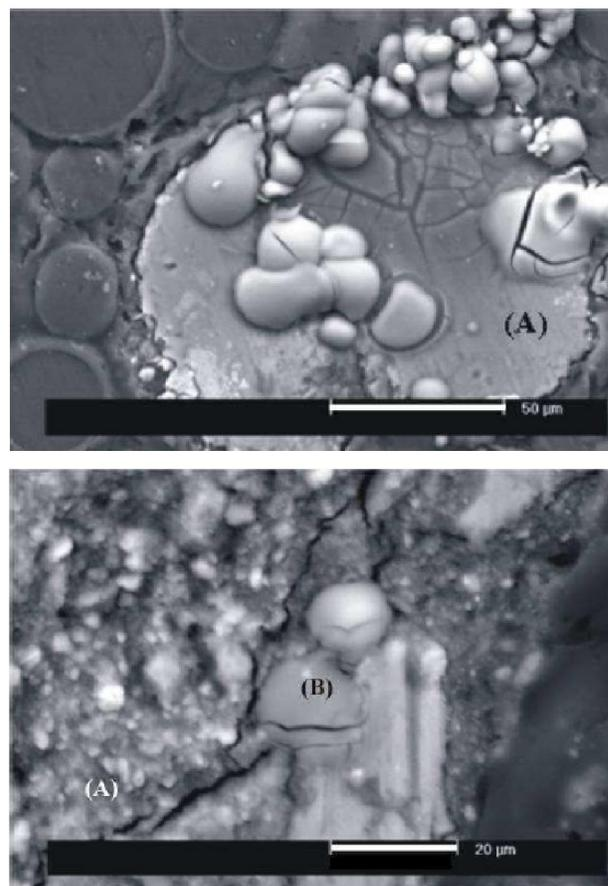
**Figure 2 :** SEM micrographs of dross samples a) before and b) after washing procedure.
