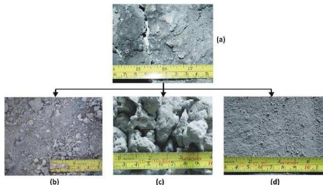
**Figure 1 :** Sequence of dross sample treatment: a) As-received, b) Milled c) Collected aluminum in ball milling, and d) Dross sieved to -12 mesh.
