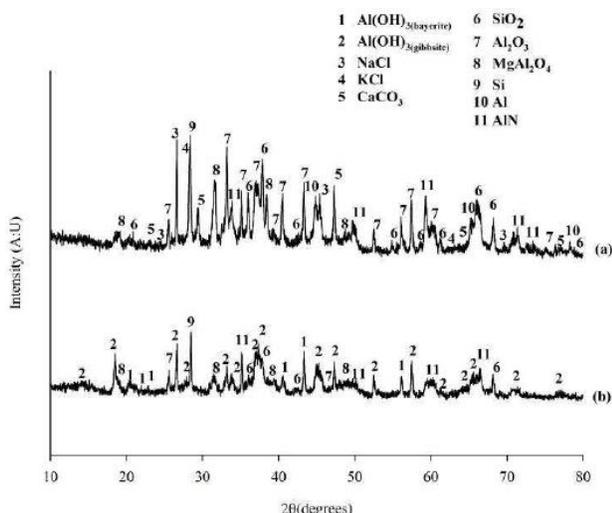
Figure 3 : X-ray diffraction pattern of a dross sample: a) as received, b) after washing process.
