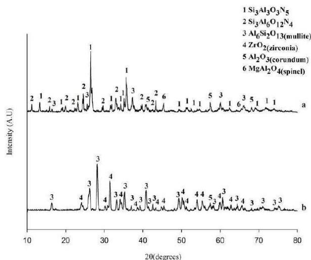
Figure 4 : XRD patterns of the synthesized ceramics: a) SiAlON composite and b) mullite-zirconia composite.
