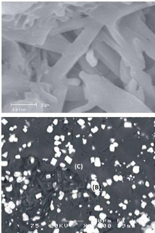
Figure 5 : SEM images of the synthesized ceramics: a) SiAlON composite and b) mullite-zirconia composite.
