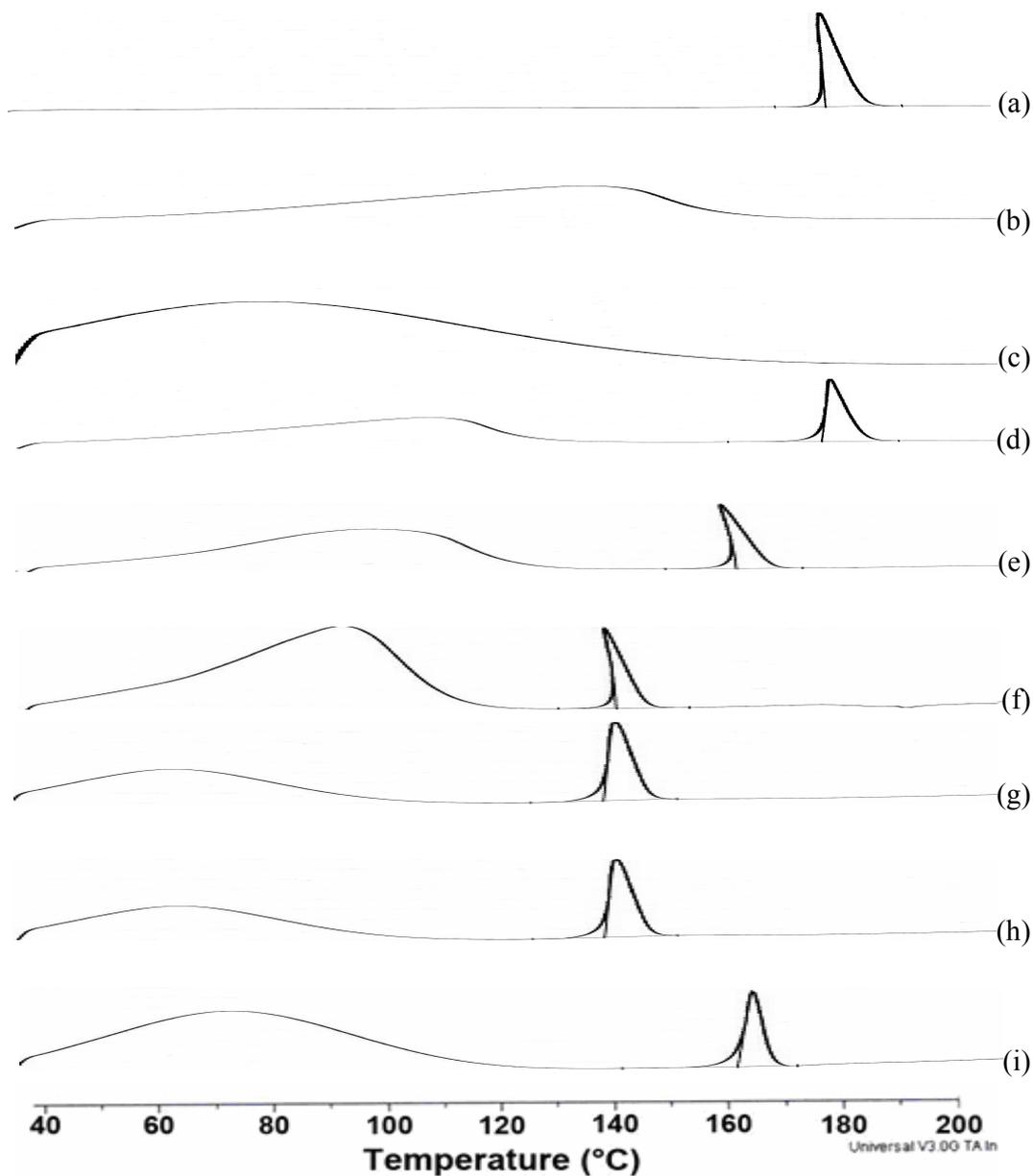
**Fig. 3:** Differential scanning calorimetry thermograms of celecoxib and its cyclodextrin complex systems. Celecoxib (a);  $\beta$ -CD (b); HP  $\beta$ -CD (c); celecoxib:  $\beta$ -CD(1:1) (d); celecoxib:  $\beta$ -CD(1:2) (e); celecoxib:  $\beta$ -CD(1:3) (f); celecoxib:HP $\beta$ -CD(1:1) (g); celecoxib: HP $\beta$ -CD(1:2) (h); celecoxib: HP $\beta$ -CD(1:3) (i);
