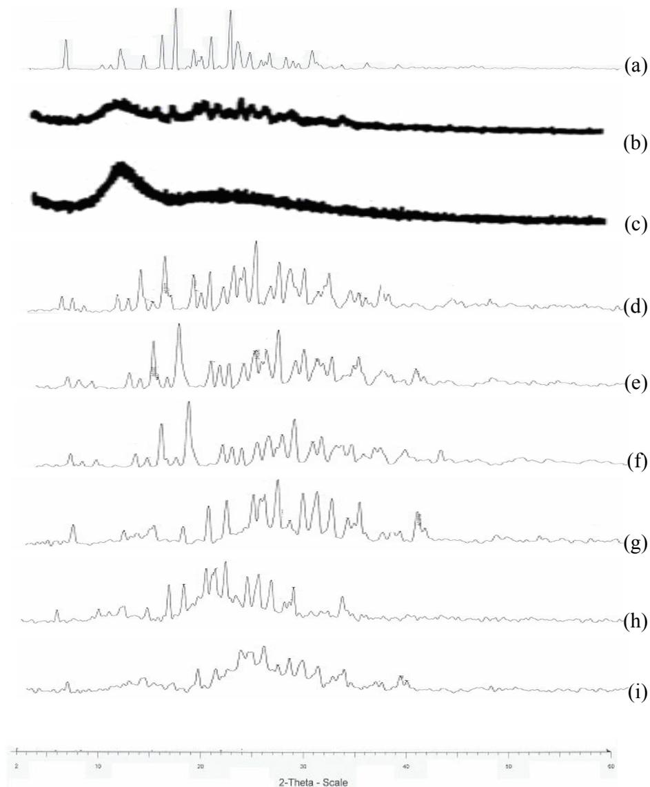
**Fig. 4: X-Ray diffractograms of powder samples of celecoxib and its cyclodextrin complex systems. Celecoxib (a);  $\beta$ -CD (b); HP  $\beta$ -CD (c); celecoxib:  $\beta$ -CD(1:1) (d); celecoxib:  $\beta$ -CD(1:2) (e); celecoxib:  $\beta$ -CD(1:3) (f); celecoxib:HP $\beta$ -CD(1:1) (g); celecoxib: HP $\beta$ -CD(1:2) (h); celecoxib: HP $\beta$ -CD(1:3) (i);**
