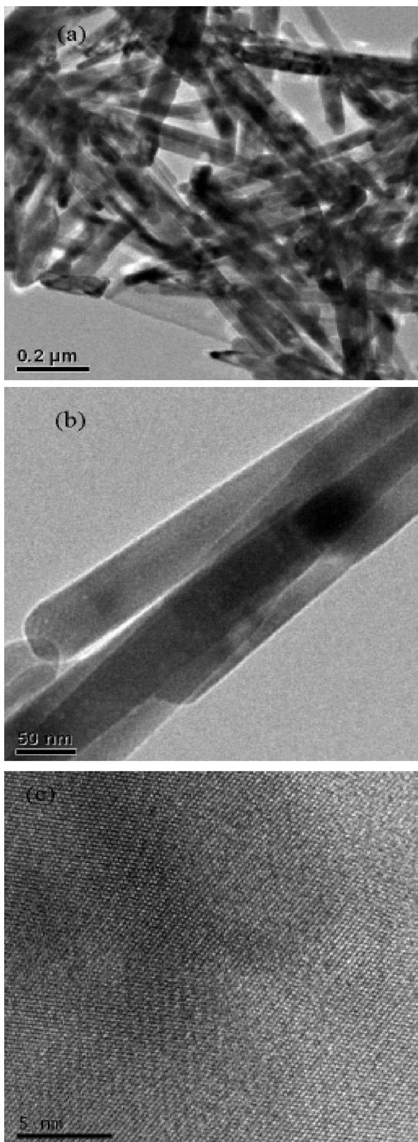
**Figure 3 :** TEM images of ZnO nanorods obtained at low citrate concentration (a) low magnification (b) high magnification (c) high resolution TEM
