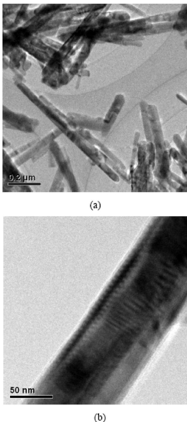
**Figure 4 :** TEM images of ZnO nanorods obtained at high citrate concentration (a) low magnification (b) high magnification
