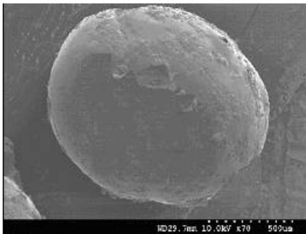
**Fig. 1: SEM of ethylene vinyl acetate copolymer (EVA) microcapsules, EVAMC1, (size 10/20) of pioglitazone**
