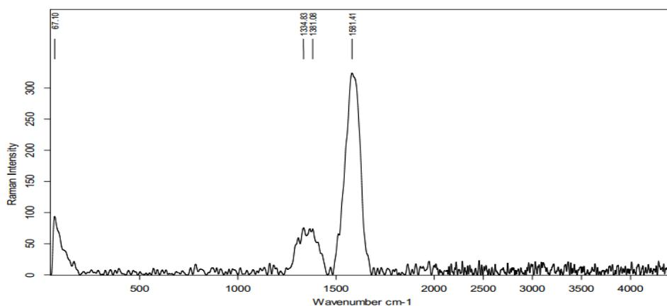
FIG. 2. Raman analysis of prepared ACTF.
