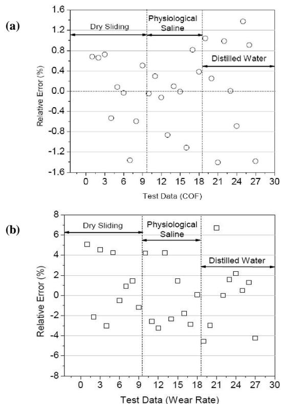
**Figure 8 :** Relative error distribution obtained from the developed ANN network as a function of the test (a) coefficient of friction data and (b) wear rate data.
