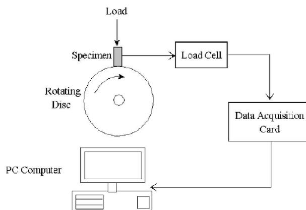
Figure 1 : Schematic diagram showing the pin-on-ring wear tester.
