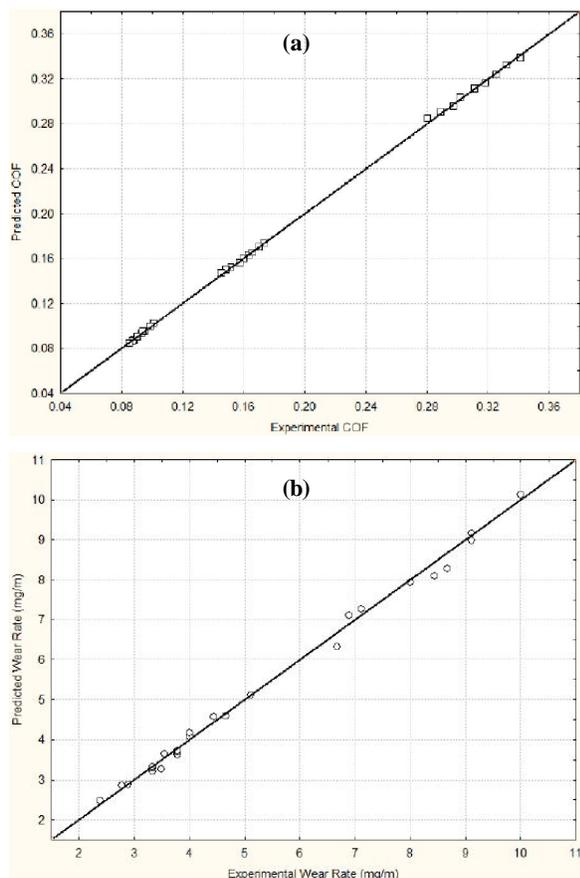
**Figure 7 :** Predicted values from the developed ANN model versus the experimental values of both (a) the coefficient of friction and (b) the wear rate of UHMWPE.
