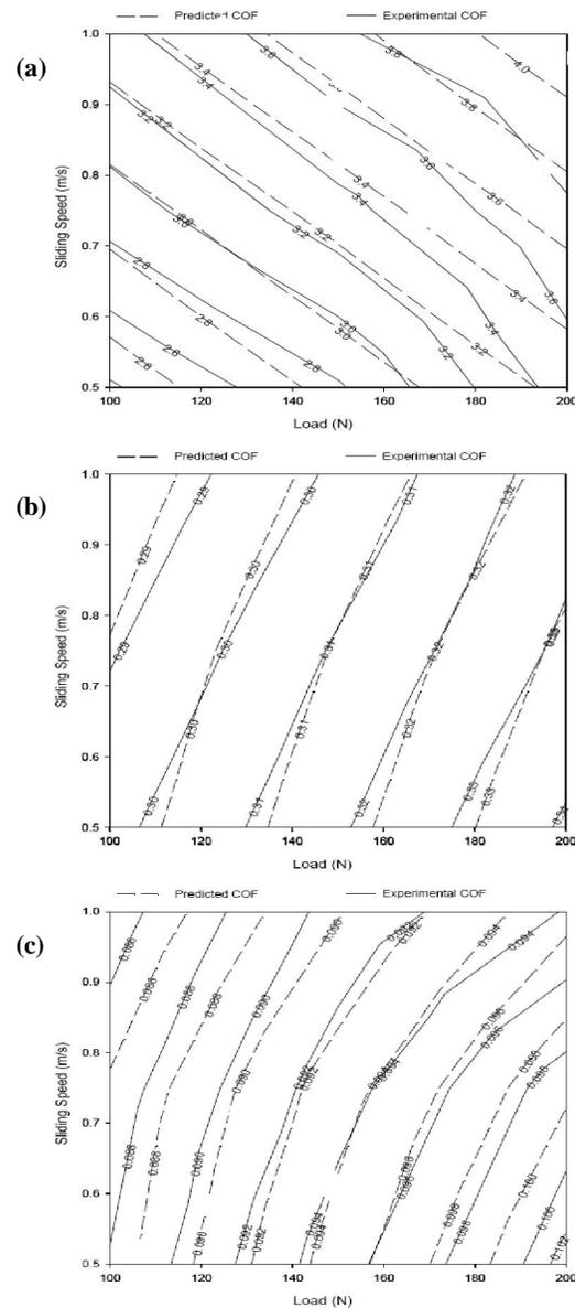
**Figure 10 :** Contour plot of the experimental and predicted coefficient of frictions of UHMWPE as a function of the applied load and sliding speed under (a) dry sliding, physiological saline (b) and distilled water (c) lubrication.
