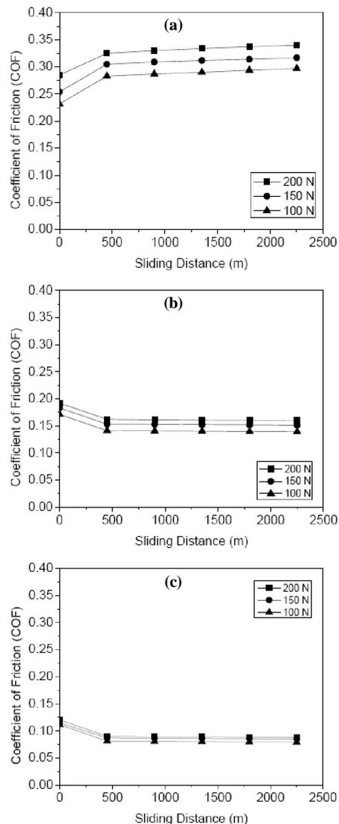
Figure 3 : Variation of friction coefficient with sliding distance at  $V=1(m/s)$  (a) (dry) (b) Under physiological saline lubricated condition (c) under distilled water lubricated condition
