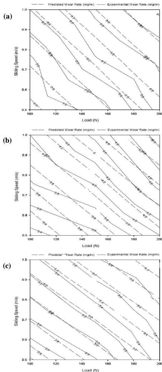
**Figure 9 :** Contour plot of the experimental and predicted wear rates of UHMWPE as a function of the applied load and sliding speed under (a) dry sliding, physiological saline (b) and distilled water (c) lubrication.
