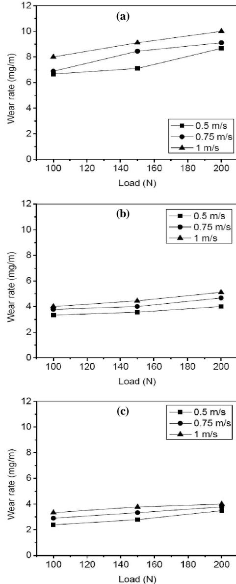
Figure 6 : Variation of wear rate with both the applied load and sliding speed under dry (a), physiological saline (b) and water (c) lubricated conditions.
