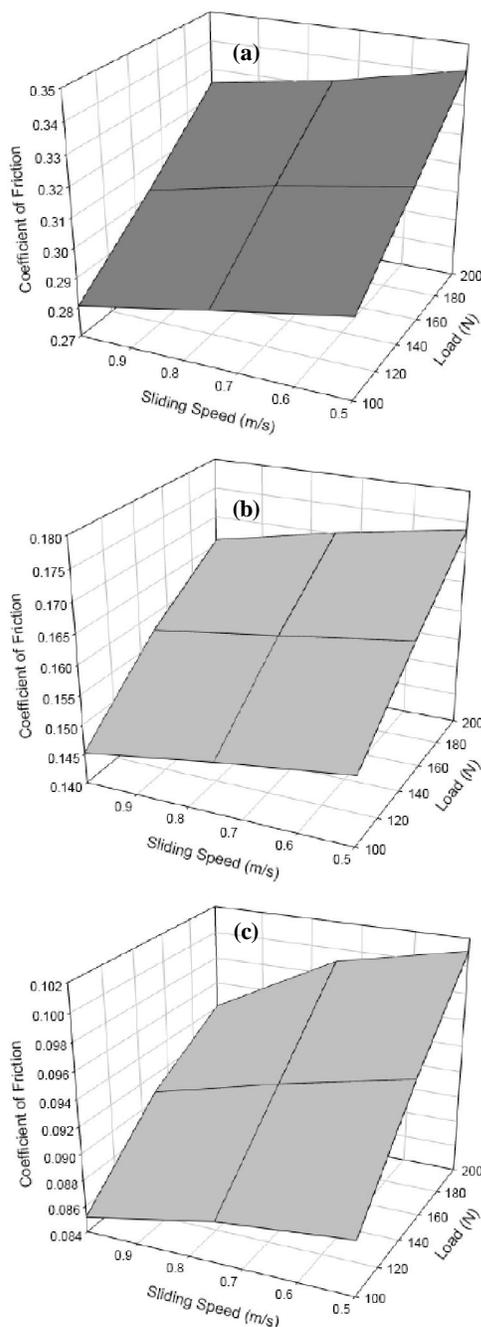
**Figure 4 :** Three dimension plots showing the variation of friction coefficient with both the applied load and sliding speed under dry (a), physiological saline (b) and water (c) lubricated conditions.
