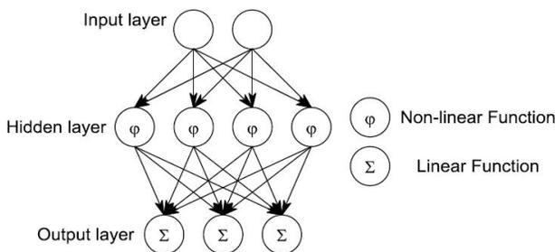
Figure 2 : Signal-flow graph of an MLP network.
