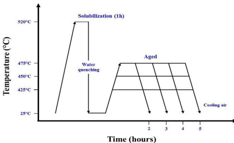
Figure 1 : Diagram showing the heat treatment to which samples were subjected, to obtain the maximum hardness as a function of time and temperature.
