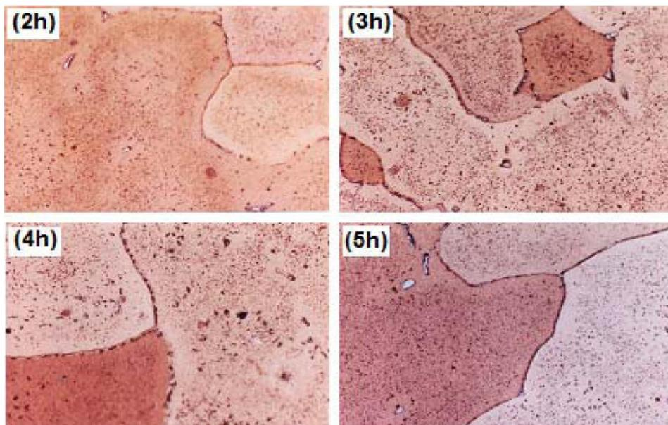
**Figure 4 :** Microstructure of sample aged at 450°C during different times.
