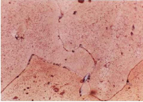
**Figure 2 :** Microstructure of ASTM-B534 alloy. Solubilized at 920°C for 1 hour.
