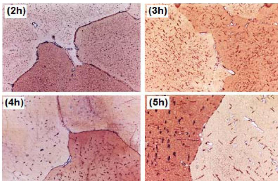
**Figure 5 : Microstructure of sample aged at 475°C during different times.**
