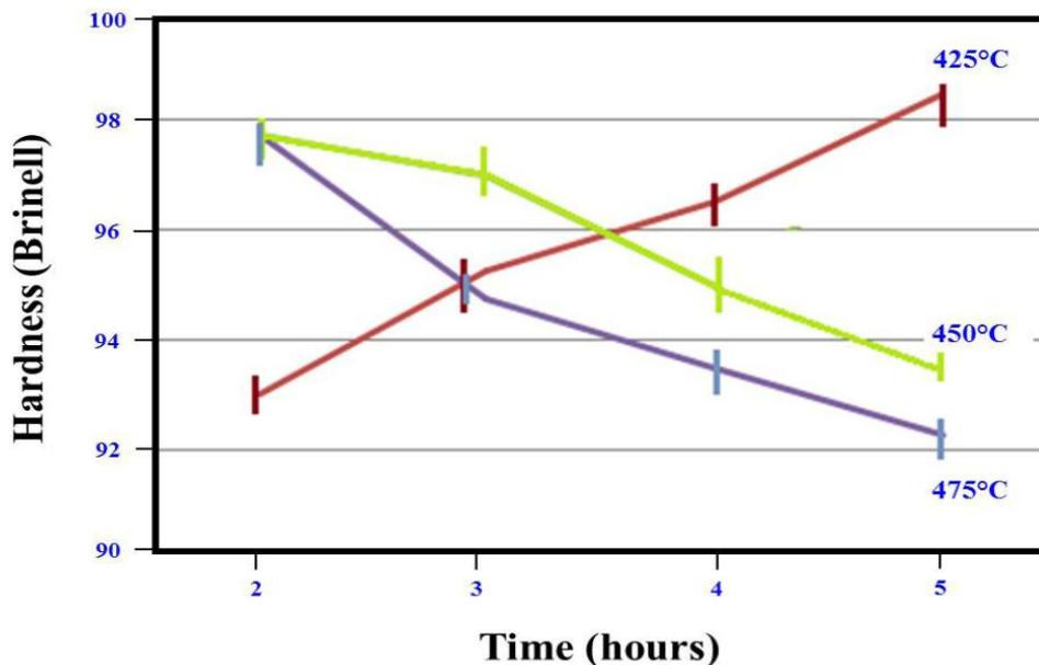
Figure 6 : Hardness of the aged samples at different temperatures depending on the aged time.
