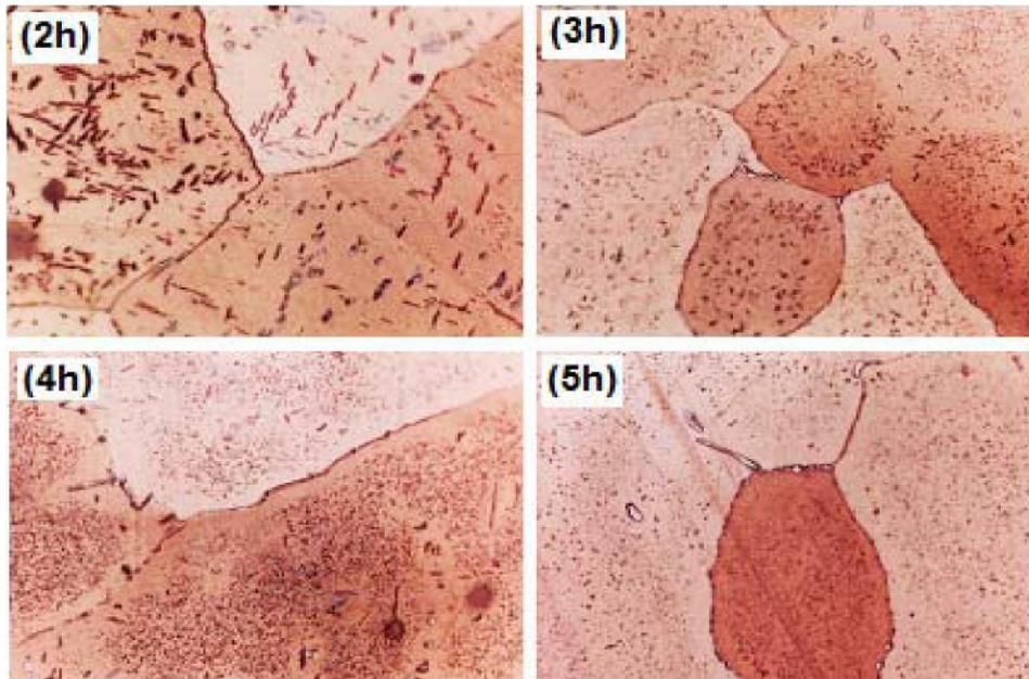
**Figure 3 :** Microstructure of sample aged at 425°C at different times.
