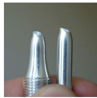
Figure 4 : Ruptured tensile specimen
