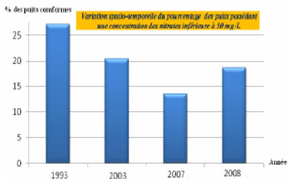
Figure 4 : Variation of the percentage of the wells having a nitrate concentration inferior to 50mg /L in function of time
