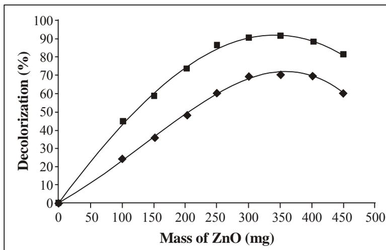
**Fig. 3: Mass effect of ZnO on decolorization of simulated textile industrial wastewater**
