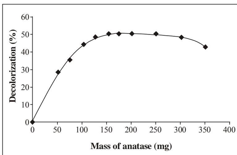
**Fig. 2: Effect of mass of anatase on decolorization % of real textile industrial wastewater**
