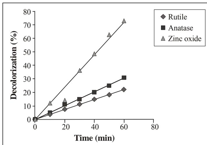
**Fig. 4: Decolorization percentage of real textile industrial on wastewater on different catalysts**
