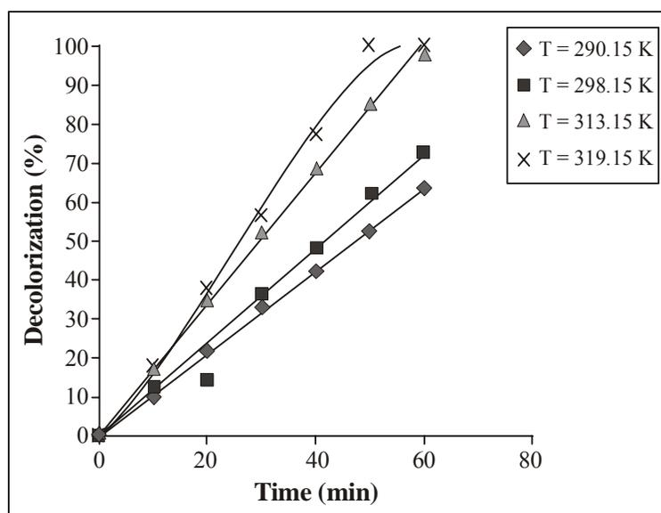
**Fig. 7: Effect of temperature on decolorization efficiency**
