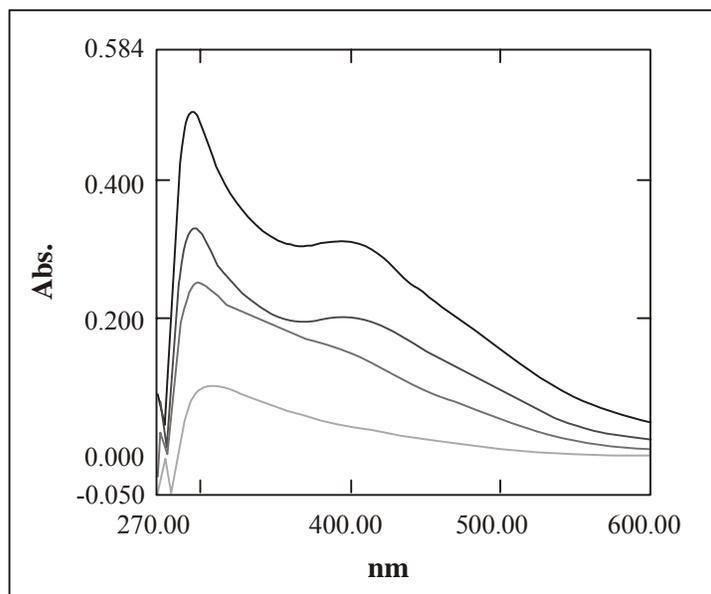
**Fig. 5: UV-Visible spectra of decolorization of real textile industrial wastewater after 60 minutes of irradiation for different initial dye concentrations on anatase at 298 K**
