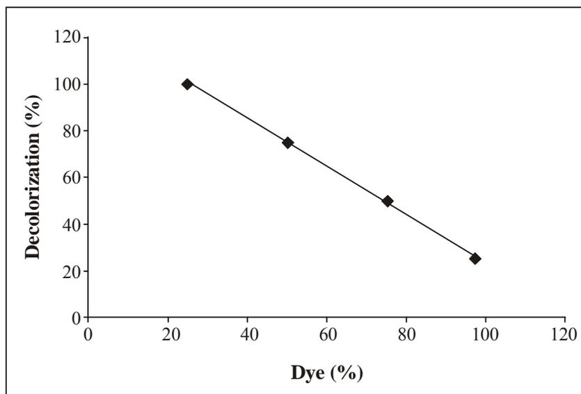
**Fig. 6: The change of decolorization percentage of real textile industrial wastewater and initial dye concentrations on anatase at 298 K.**
