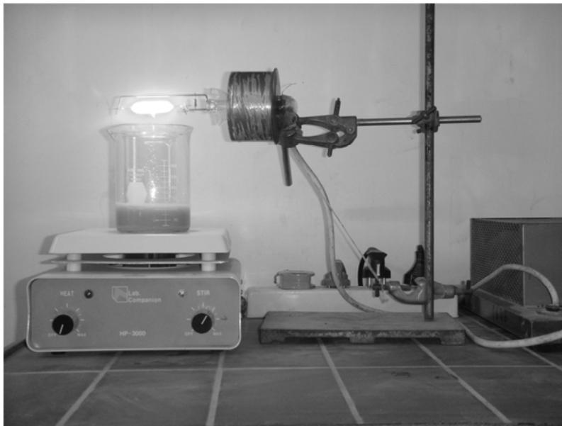
**Fig. 1: Photocatalytic reactor**
