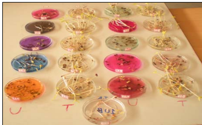
Fig. 3: The effect of treated and untreated dye water on the number of seed germination
