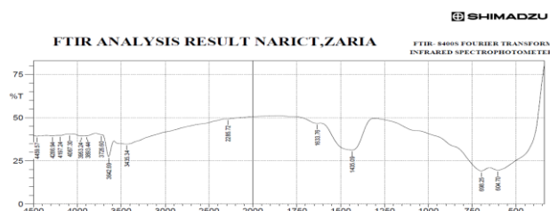
FIG. 9. FT-IR spectrum of used 1% Zn-TiO 2 after the photodegradation.
