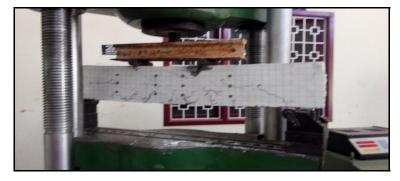
Fig. 10: Crack pattern
