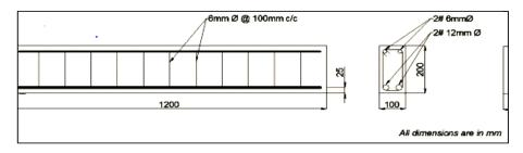
Fig. 1: Beam reinforcement details
