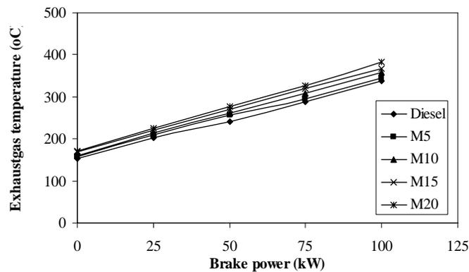
**Fig. 5: Exhaustgas temperature Vs brake power**
