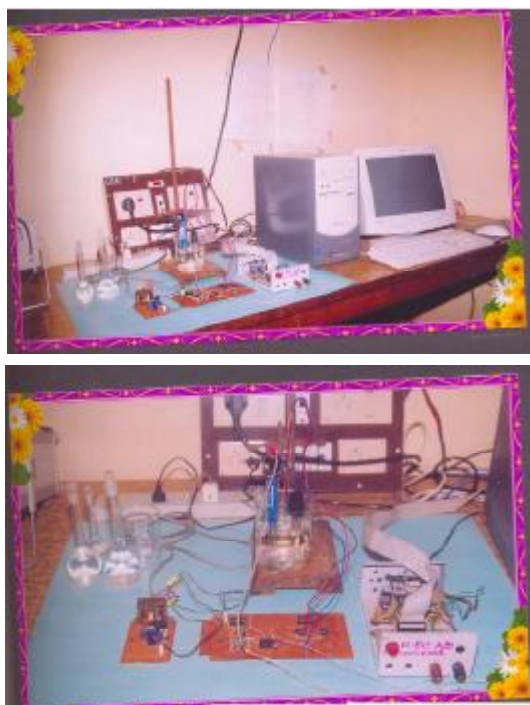
Figure 2: The complete photograph of PC based system for conductivity measurement.
