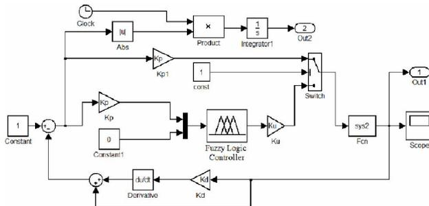
**Figure 8 : Simulink block diagram of optimal DFPD simulation**
