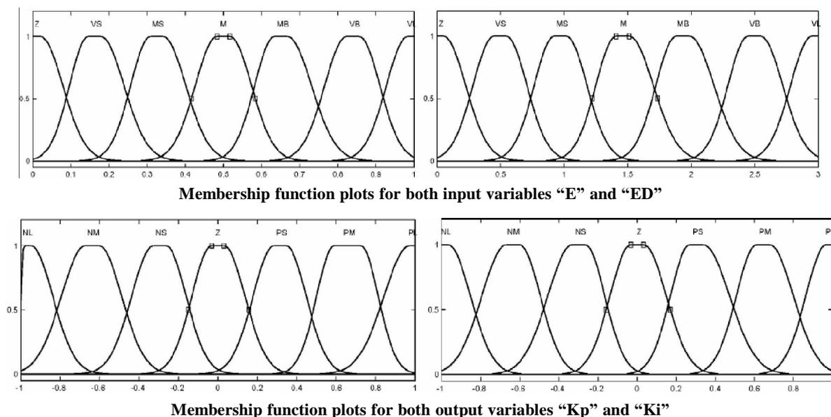
Figure 2 : Membership function plots for both input variables and output variables
