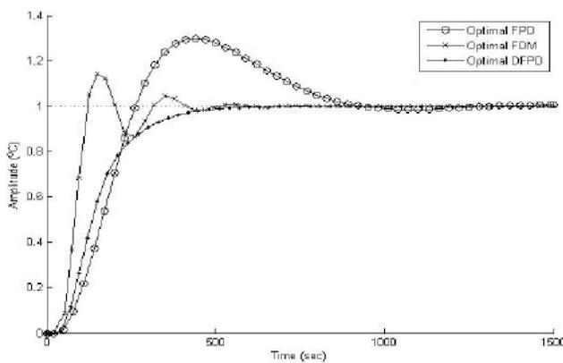
**Figure 7 : The Unit step responses of different optimal fuzzy PD controllers**
