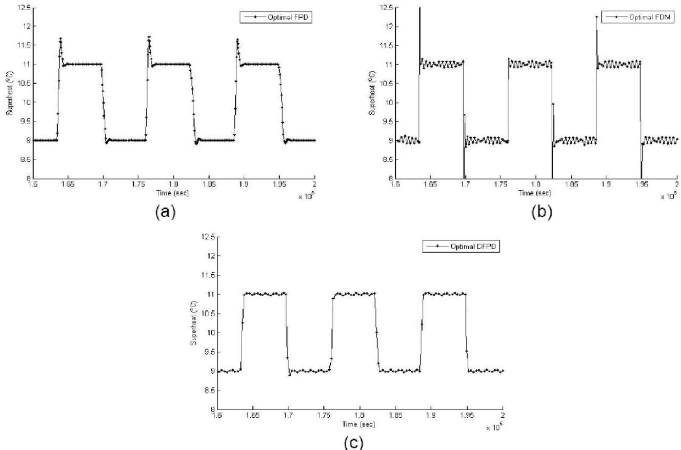
**Figure 9 : Superheat response of evaporator based on optimal fpd controller(a), optimal fdm controller(b), and optimal dfpd controller(c), respectively**
