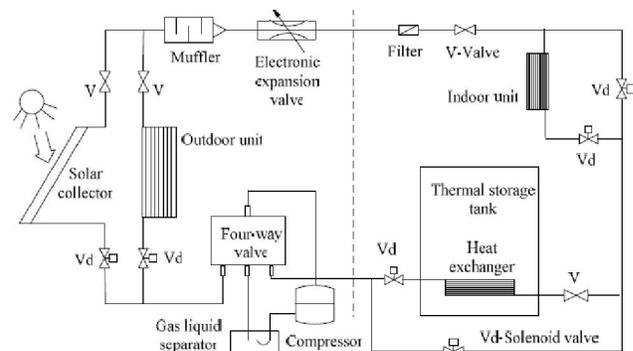
Figure 1 : Basic schematic diagram of SHP testing system
