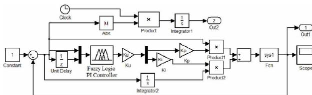
Figure 5 : Simulink block diagram of the first type system based on optimal FPI controller
