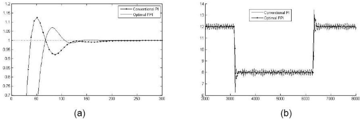
**Figure 6 : The unit step responses(a) and superheat responses(b) of optimal PI controller and conventional PI controller**
