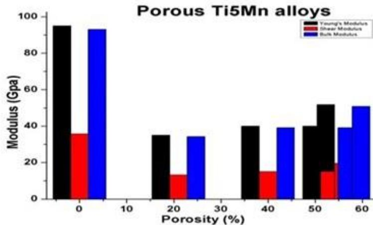
FIG. 1. Influence of porosity on Modulus of porous Ti5Mn alloys.
