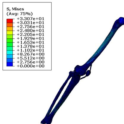
**Figure 2 : Overall stress distribution map of knee joint when standing on one leg**
