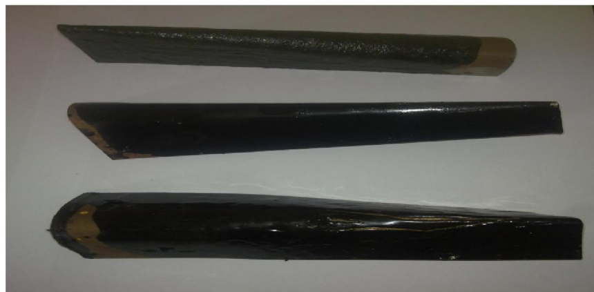
Figure (5C) : Mandrel bend testing panel of asphalt modified with 10%RNP, 3%RNP and AC virgin
