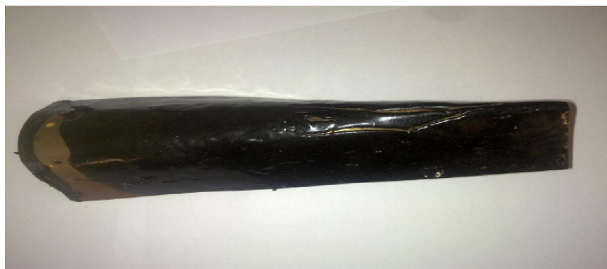
Figure (5A) : Mandrel bend testing panel of virgin asphalt
