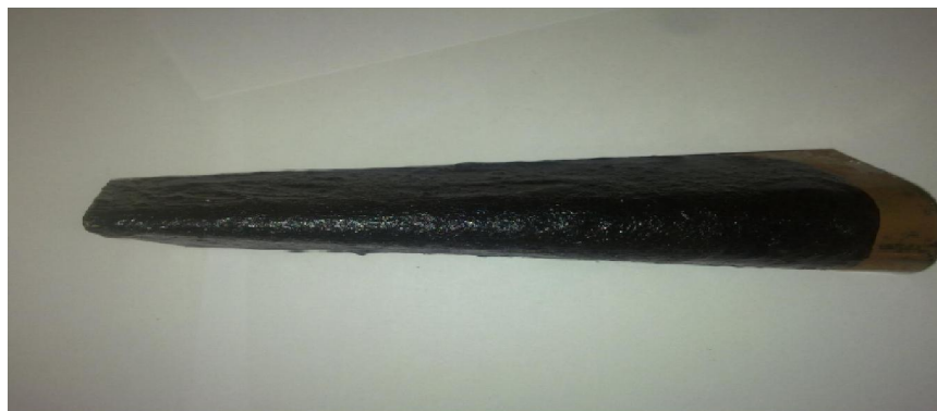
Figure (5B) : Mandrel bend testing panel of asphalt modified with 10%RNP
