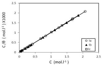
Figure 4 : Langmuir isotherm plots for carbon steel in 1M HCl at presence of different concentrations of cationic gemini surfactants Ia, Ib and Ic.
