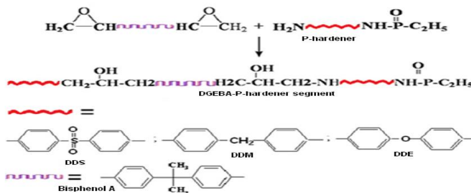
Scheme 1 : Reaction of DGEBA epoxy with P-hardeners.
