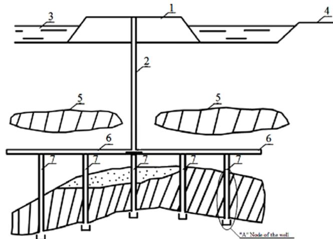
**Fig. 1: Method of opening and exploitation of offshore and onshore oil reservoirs**
