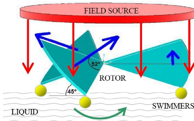
Figure 5 : Electrostatic rotor, consisting of a field source (red) and a rotor (blue)
