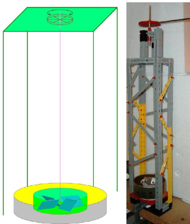
Figure 8 : The torsion balance for the measurement of the mechanical power-output.
