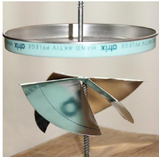
Figure 10 : Electrostatic rotor and field-source for the test of a potential recoil at the quantum-vacuum.
