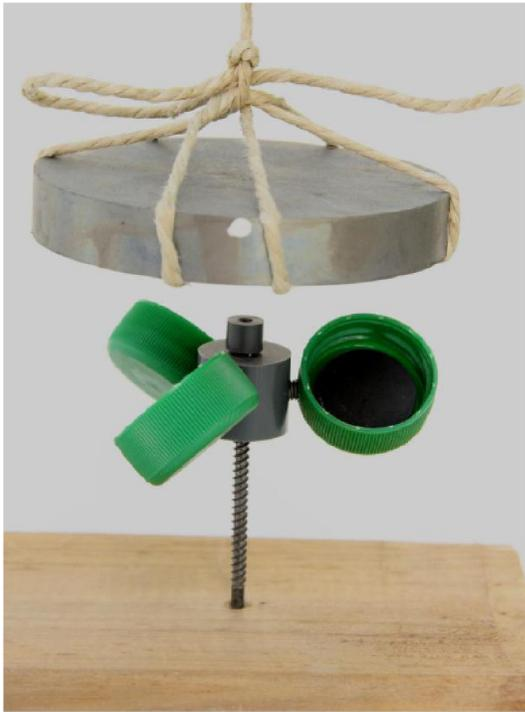
Figure 16 : Real setup of a magnetostatic rotor with rotor-blades of high- $T_c$ -superconductor, mounted under a rare earth magnet
