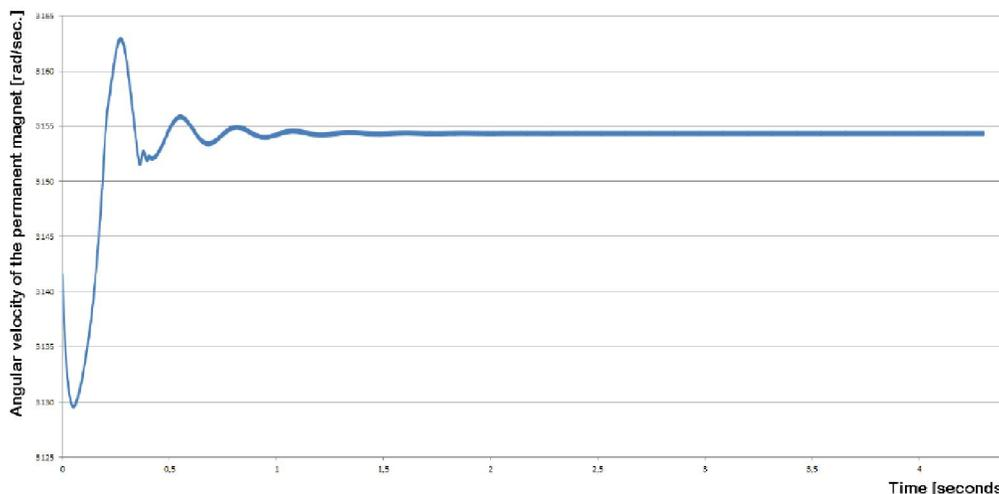
Figure 14 : Result of a theoretical computation of the angular velocity of the magnet, during the starting mode of the engine.
