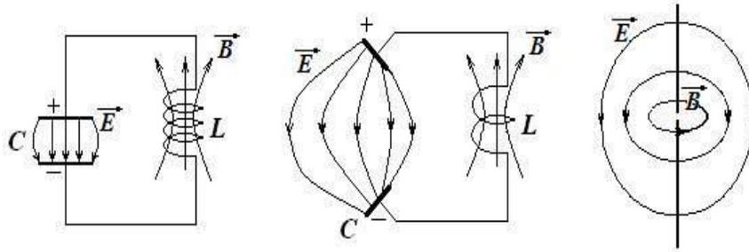
**FIG. 1. Transformation of a closed electrical oscillatory circuit into the open.**
