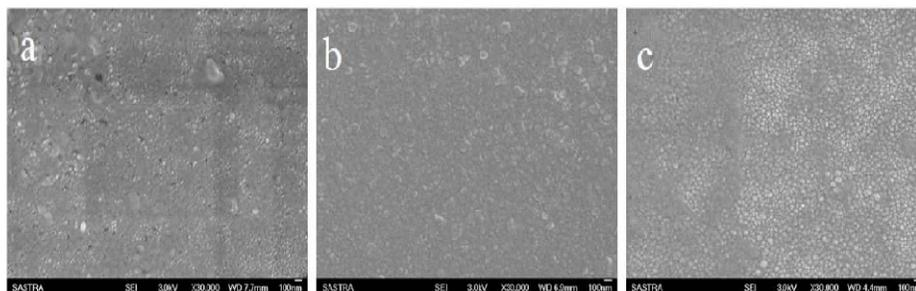
Figure 2: FE-SEM micrographs of ZnO films deposited at different cathode powers of a) 20, b) 30 and c) 40 W
