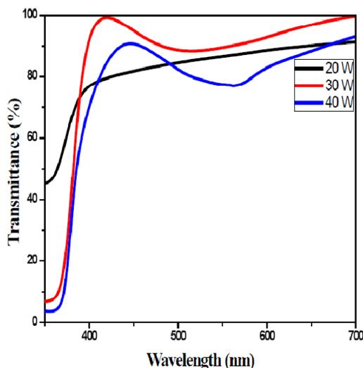
Figure 3: Optical transmittance of ZnO films deposited at different cathode powers
