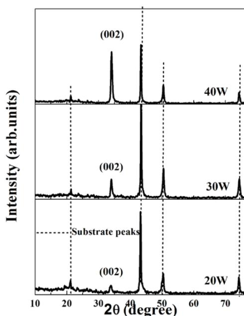
Figure 1: XRD patterns of ZnO films deposited at different cathode powers
