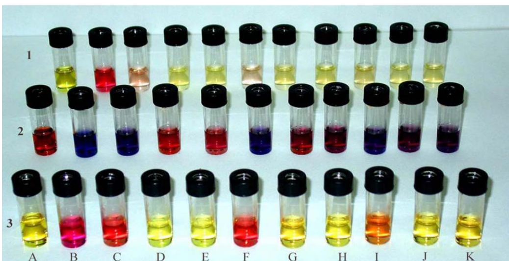
Figure 3 : Photograph showing the color of dilute solutions of 1,5-DHA (1), 1,2,5,8-THA (2) and 1,8-DHA (3) in DMS. ([quinone] = 3.3 \times 10^{-4} M) and ([anion] = 1 \times 10^{-3} M) for all excepting \text{Cl}^- , \text{Br}^- and oxalate that was 1.10^{-2} M). Files notation: A) AQ pure, B) \text{CO}_3^{2-} , C) \text{HCO}_3^- , D) \text{Cl}^- , E) \text{Br}^- , F) \text{HPO}_4^{3-} , G) \text{H}_2\text{PO}_4^{2-} , H) acetate, I) citrate, J) tartrate, K) oxalate.
