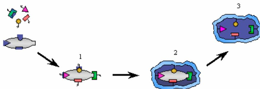
Figure 1: Schematic representation of the molecular imprinting process. (1=Assembly; 2 = Polymerisation; 3 = Template Extraction)
