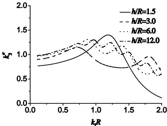
Figure 10 : Variation of DSIF vs. wave number and  $h/R$
