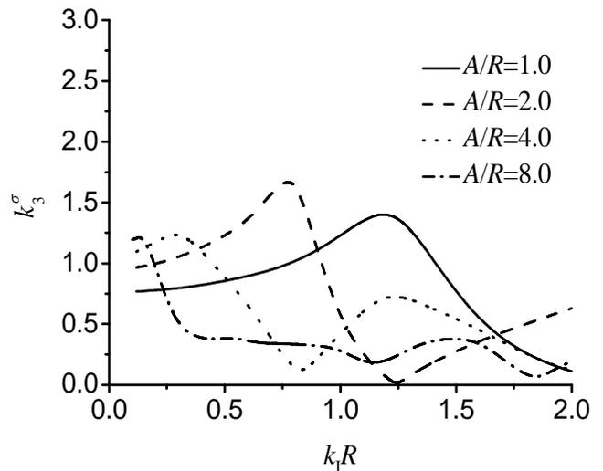
Figure 9 : Variation of DSIF vs. wave number and  $A/R$
