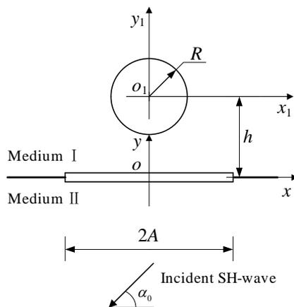
Figure 1 : Interacting interface crack and a circular cavity in a piezoelectric bimetals
