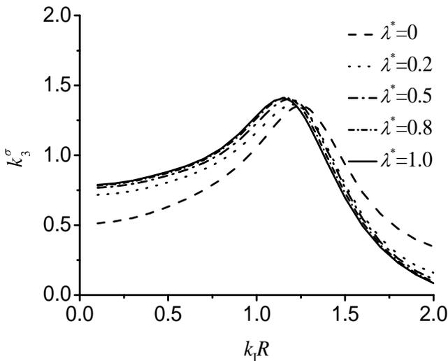
Figure 8 : Variation of DSIF vs. wave number and  $\lambda^*$
