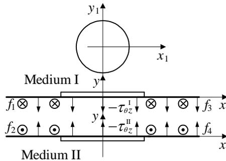
Figure 2 : Conjunction of two semi-infinite piezoelectric media
