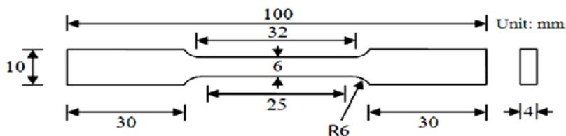
**Fig. 2: Dimensions of the tensile specimen**
