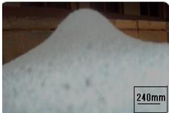
Figure 1 : Spray deposited preform
