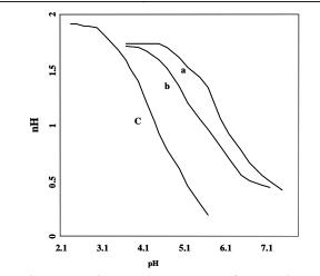
Figure 2 : protonation constantes curves of enalapril maleate at a = 0.05 M, b = 0.1 M, C = 0.15 M
