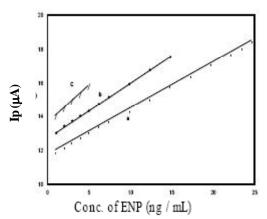
Figure 8 : Plot of Ip versus concentrations of enalapril using 0.04 M of Britton - Robinson buffer (pH~9.0) at different accumulation times: (a): 15 s (b): 30 s (c): 60 s
