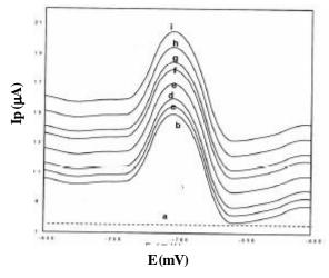
Figure 9 : Typical SWCS voltammograms of Enalapril different concentrations in presence of 0.04 M Britton - Robinson buffer (pH ~9.0) at 60 s
