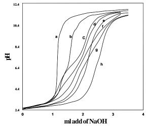
Figure 1 : Titration curves of enalapril with different metal ions at I = 0.05 M NaNO<sub>3</sub> (in aqueous - ethanolic solution) a = acid solution, b = solution (a) + ligand (ENP), c = solution (b) + Cu(II) ion, d = b + Cr(III) ion, e = b + Fe (III) ion, f = b + Hg (II) ion, g = b + Y(III) ion, h = b + Pd (II) ion
