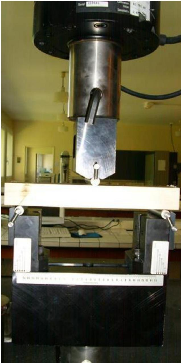
**Figure 1 :** The bending test apparatus with a raw wood sample ready to be tested
