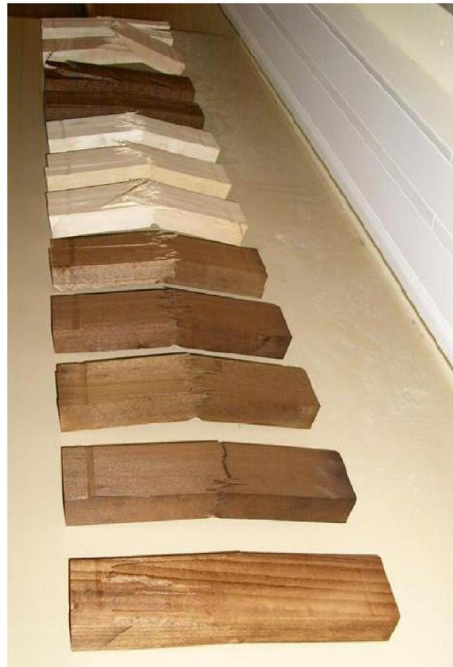
Figure 5 : Some of the raw and heat-treated beech and poplar samples after bending test
