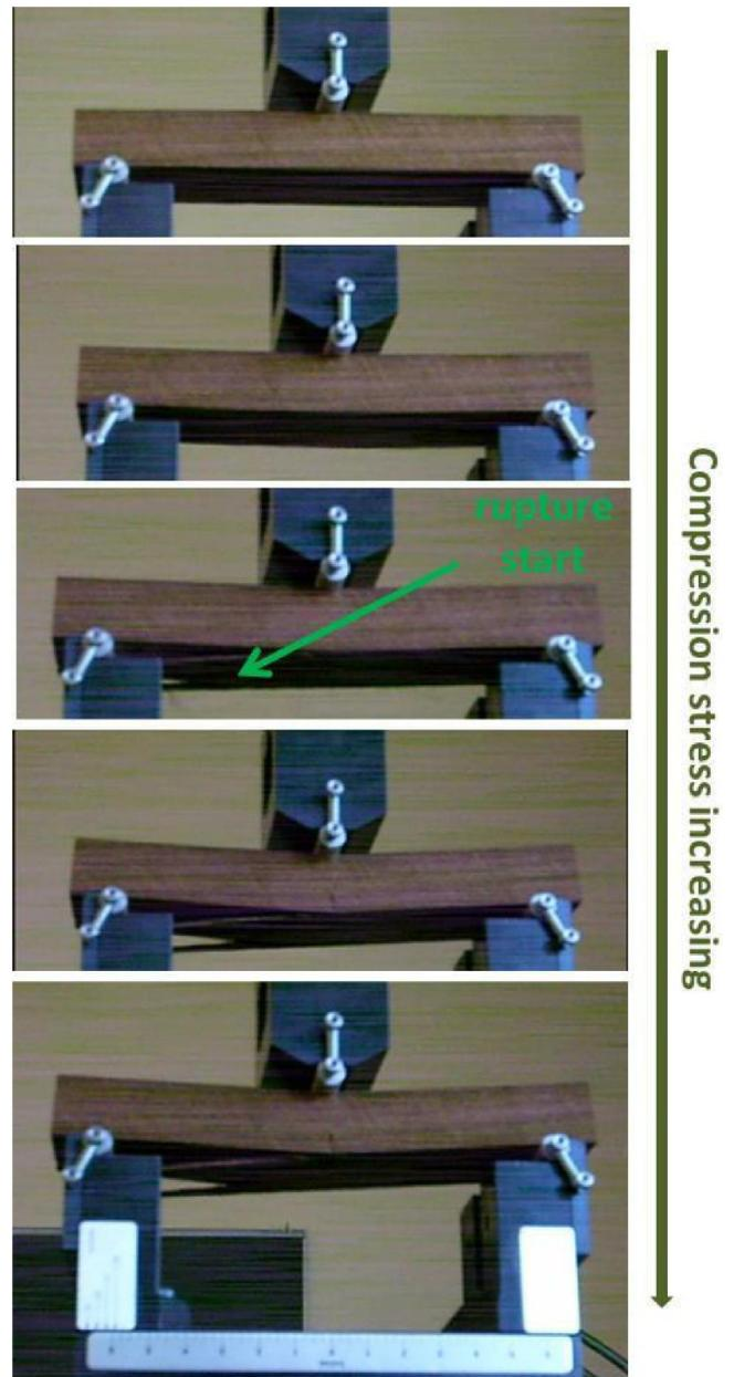
Figure 3 : Progressive deformation of a sample during bending test
