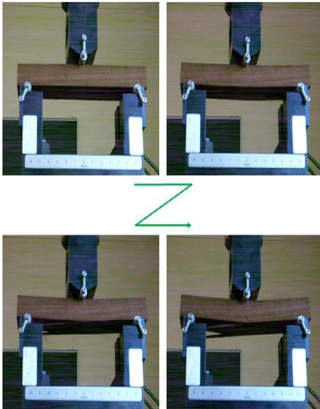
Figure 2 : Successive views of the bending test of one of the wood samples; (here: heat-treated wood)
