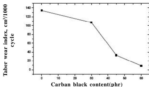
**Figure 3 : Change in the taber wear index as a function of the CB content of the SBR vulcanizates**
