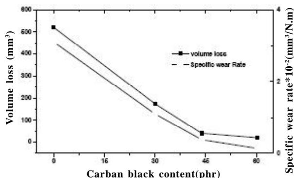
**Figure 2 : Volume loss (v) and specific wear rate (k) as a function of CB content of the SBR vulcanizates**
