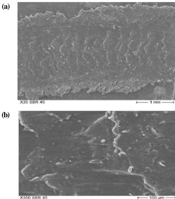
**Figure 5 : SEM worn surfaces for unfilled SBR vulcanizates at two different magnification modes**
