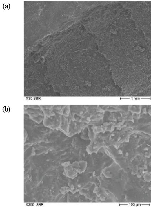
**Figure 4 : SEM worn surfaces for unfilled SBR vulcanizates at two different magnification modes**
