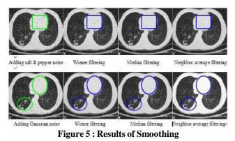
For the "Salt and Pepper" noise image, Median filtering not only filtered the noise, but also had a good effect on smoothing the image as the blue square frame showed. The Wiener filtering was not satisfactory for filtering all the sparkles completely, while the Neighbor average filtering resulted in a roughness side effect in the image.
