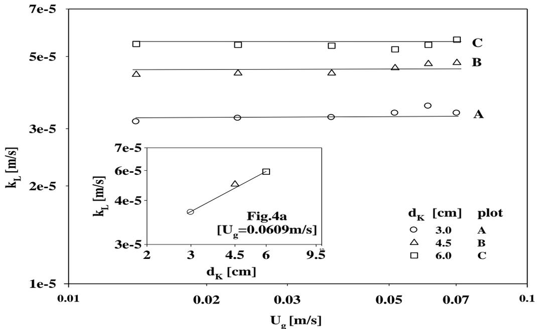
Figure 4: Variation of  $k_L$  with disc diameter for  $d_r = 10$  cm,  $p = 5$  cm,  $\theta = 45^\circ$ ,  $U_L=0.168$  m/s.
