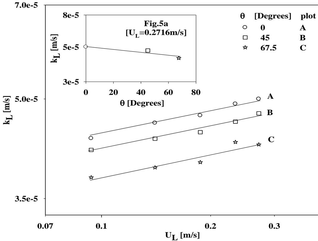
Figure 5: Variation of  $k_L$  with disc angle for  $d_r = 1.0$  cm,  $d_K = 4.5$  cm,  $p = 5$  cm,  $U_g = 0.0327$  m/s.
