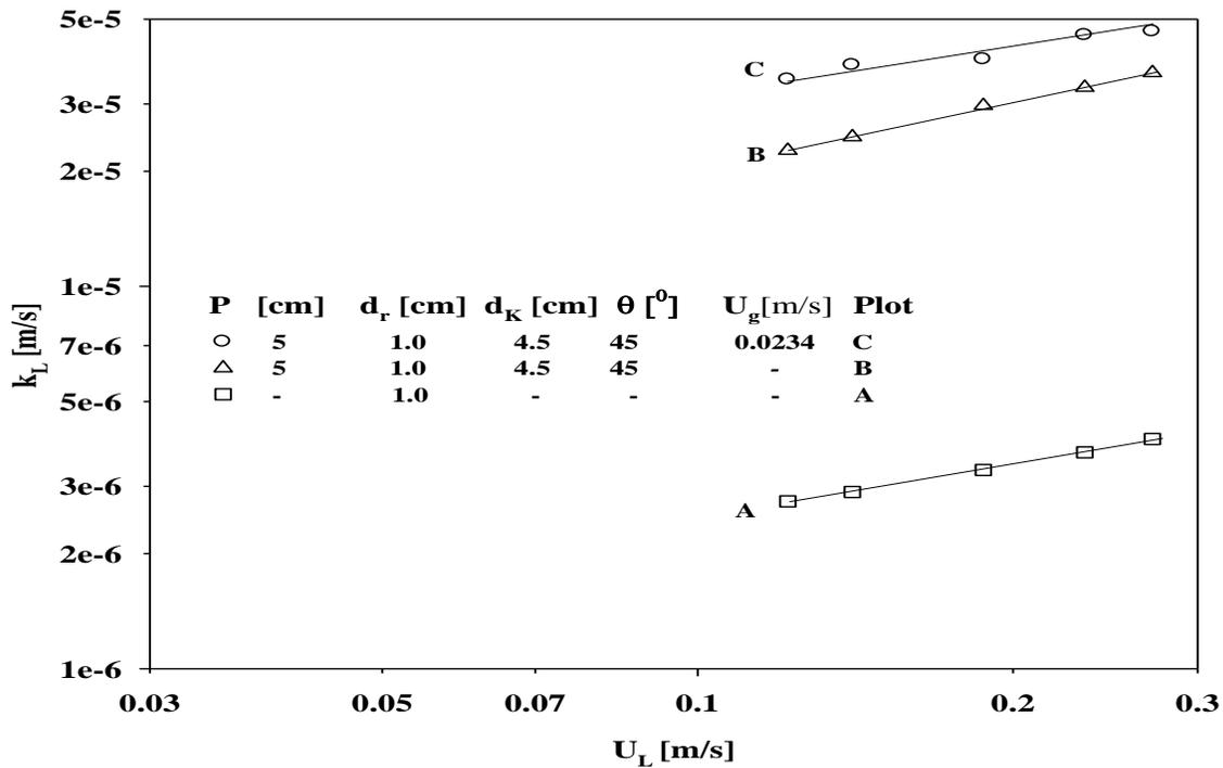
**Figure 2:** Augmentation of mass transfer coefficient with angled disc promoter.
