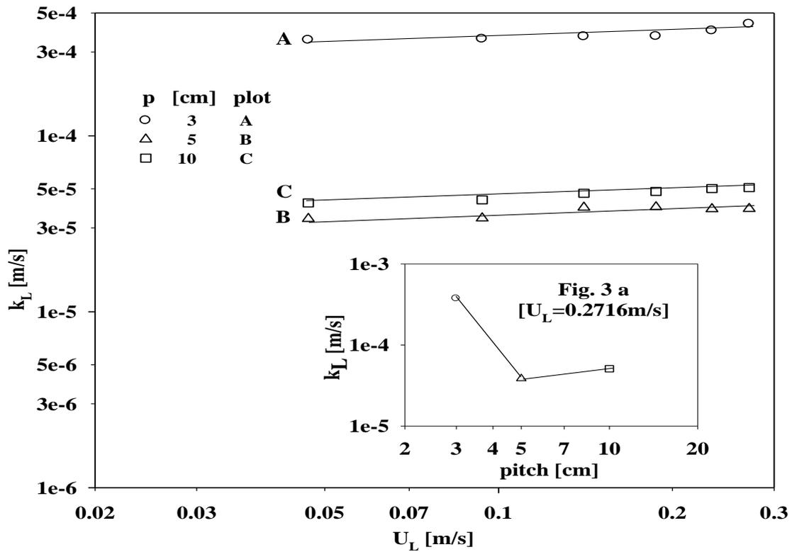
Figure 3: Variation of  $k_L$  with pitch for  $d_r = 1.0$  cm,  $d_k = 4.5$  cm,  $\theta = 45^\circ$ ,  $U_L=0.0936$  m/s.
