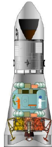
Figure 6 : The LASS within the Saturn V nose fairing with a service module for Lunar orbit insertion.
