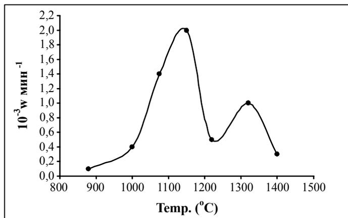
**Fig. 2: Dependence of the metal reduction speed on the temperature**
