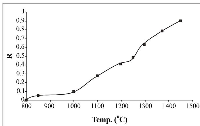
**Fig. 1: Change in ratio of reduction of the metals made of chromite ore depending on system temperature**
