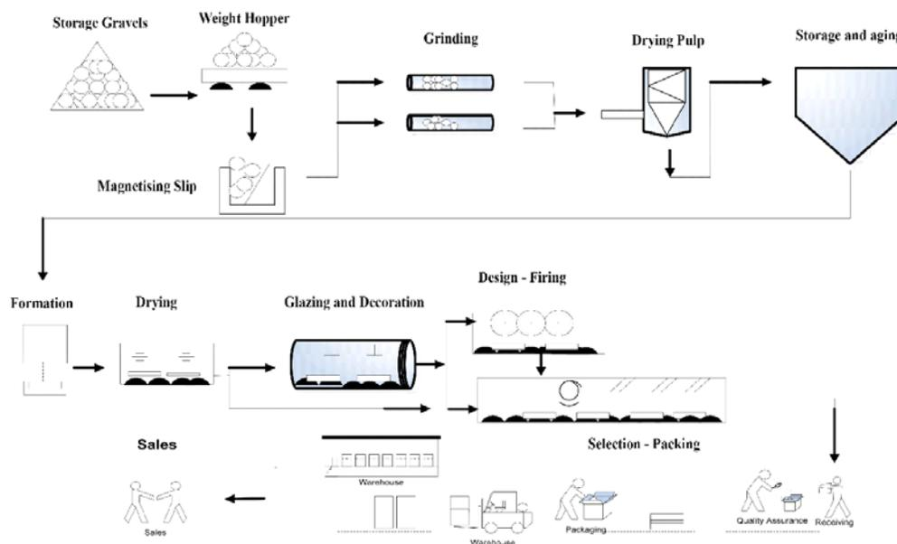
Fig. 1: Tile production flow
