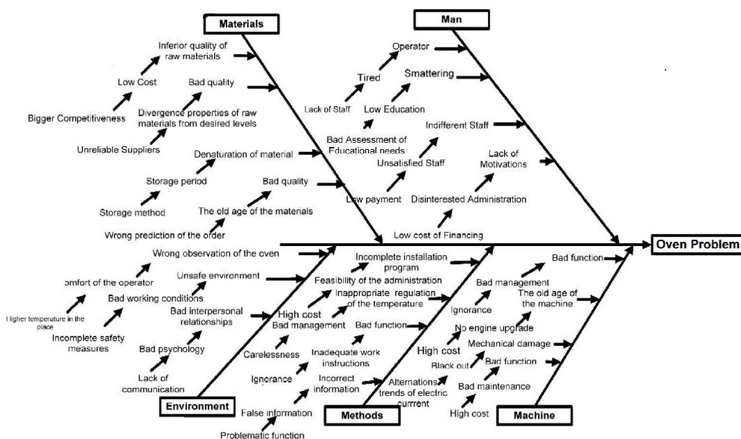
**Fig. 7: Fish bone diagram for Klin Oven**
