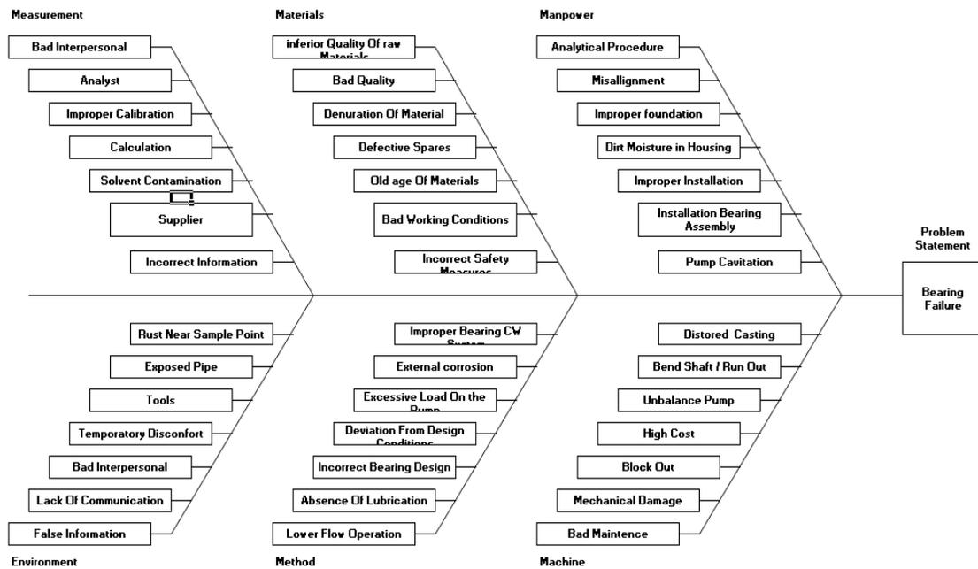
**Fig. 3: Fish bone diagram for bearing failure**
