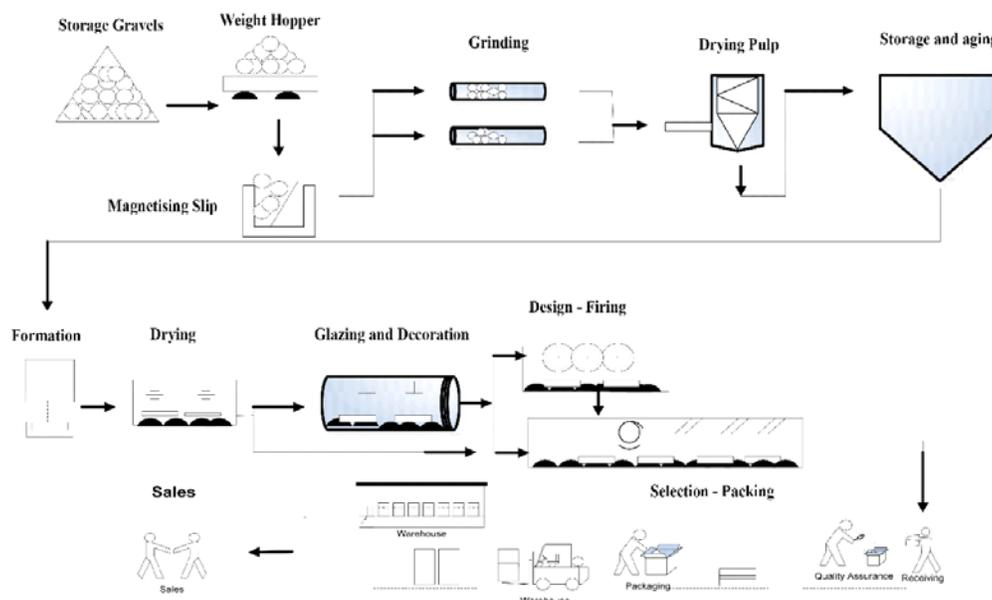
Fig. 1: Tile production flow
