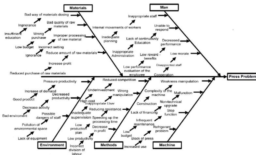
Fig. 4: Fish bone diagram for hydraulic press
