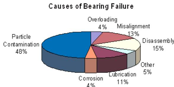
**Fig. 2: Bearing failure**
