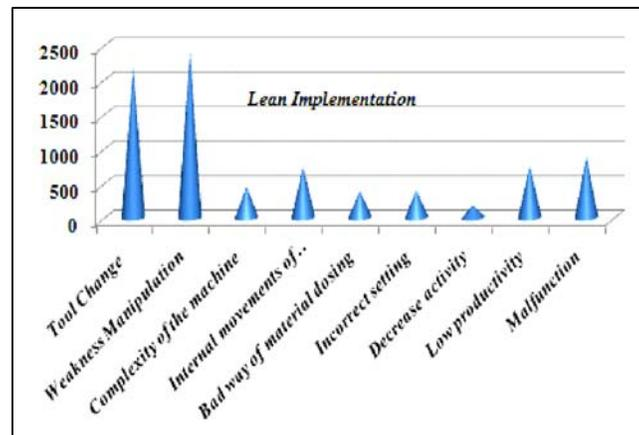
**Fig. 6: Data collection and analysis for hydraulic oven after lean implementation**
