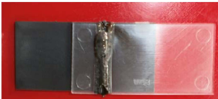
Figure 5 : welding 20~30mm/s, laser power 40W, slight degradation of the weld joint occur
