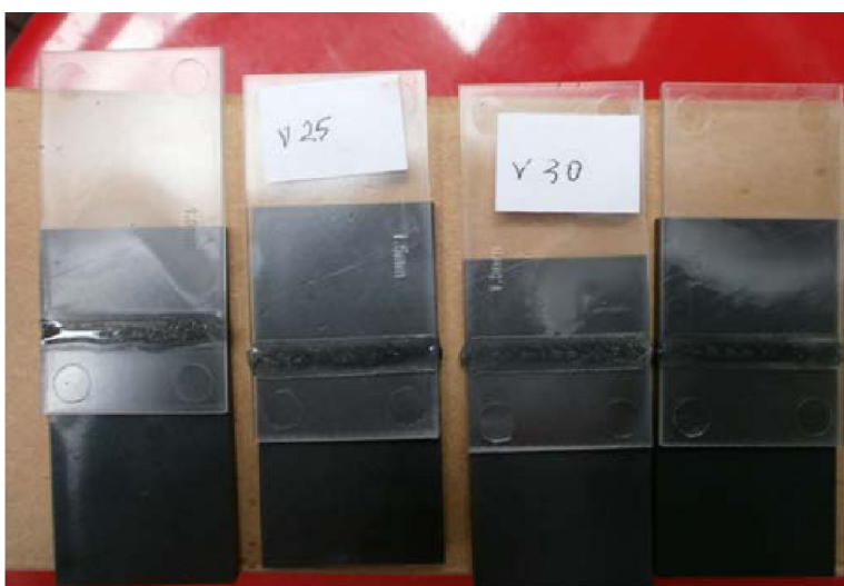
Figure 4 : welding 10mm/s, laser power 40W, overheating degradation of the weld joint occur
