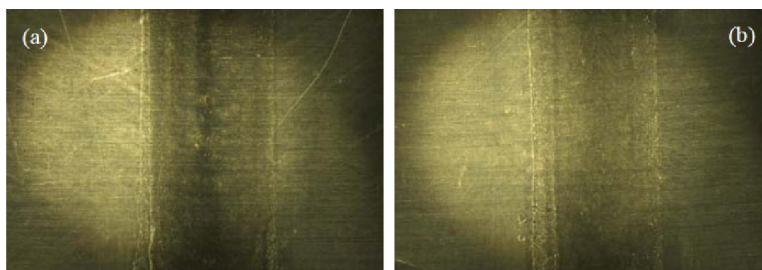
Figure 11 : Weld interface for PC with laser power 40 W, welding speed of 50mm/s; (a) transparent thickness 1mm; magnification 20 X; (b) transparent thickness 1.5mm; magnification 20 X
