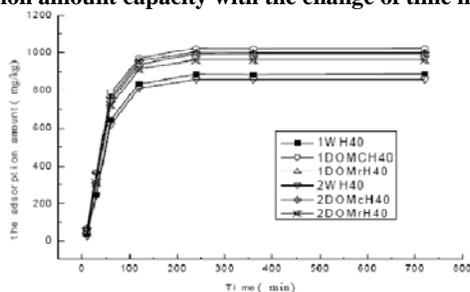
Figure 2 : Hg adsorption amount capacity with the change of time in the higher Hg content
