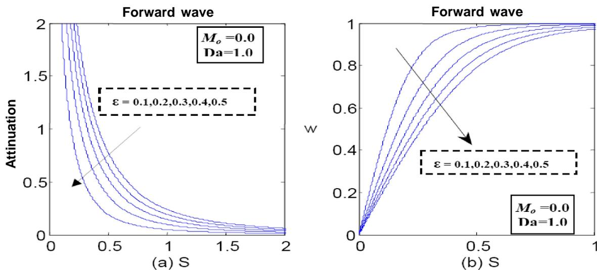
Figure 2 : Attenuation and phase shift of stationary ( $M_o=0$ ) fluid in plain media ( $Da=1$ ) at various porosity ( $\varepsilon$ ): (a) attenuation (b) phase shift
