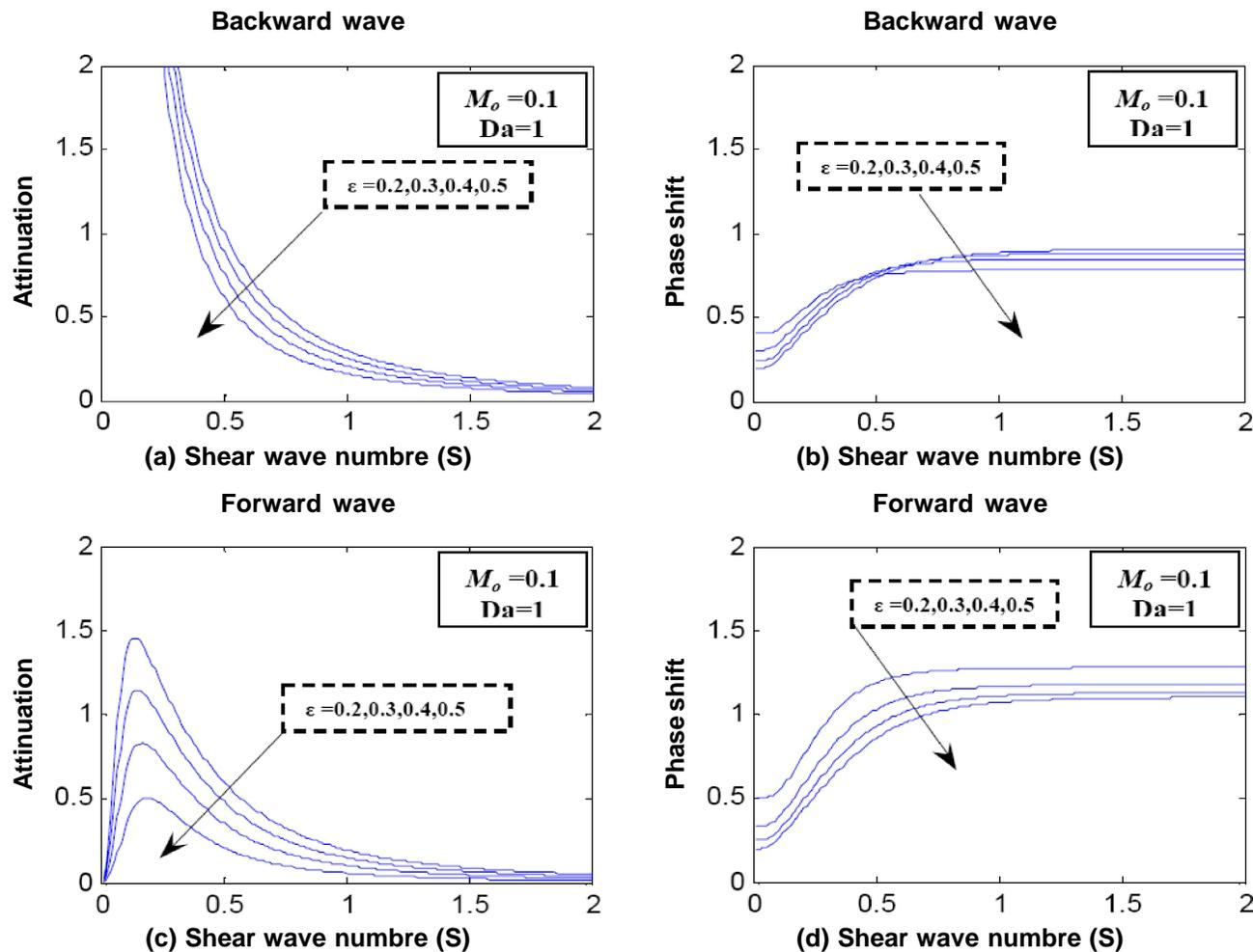
Figure 3 : Forward and backward waves attenuation and phase shift at steady state flow ( $M_o=0.1$ ) and plain media ( $Da=1$ ): (a) backward wave attenuation (b) backward wave phase shift (c) forward wave attenuation (d) forward wave phase shift
