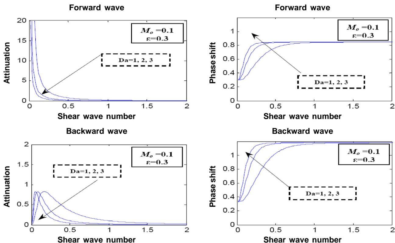
Figure 5 : Forward and backward waves attenuation and phase shift at steady state flow ( $M_o=0.1$ ) and porosity ( $\epsilon=0.3$ ): (a) backward wave attenuation (b) backward wave phase shift (c) forward wave attenuation (d) forward wave phase shift
