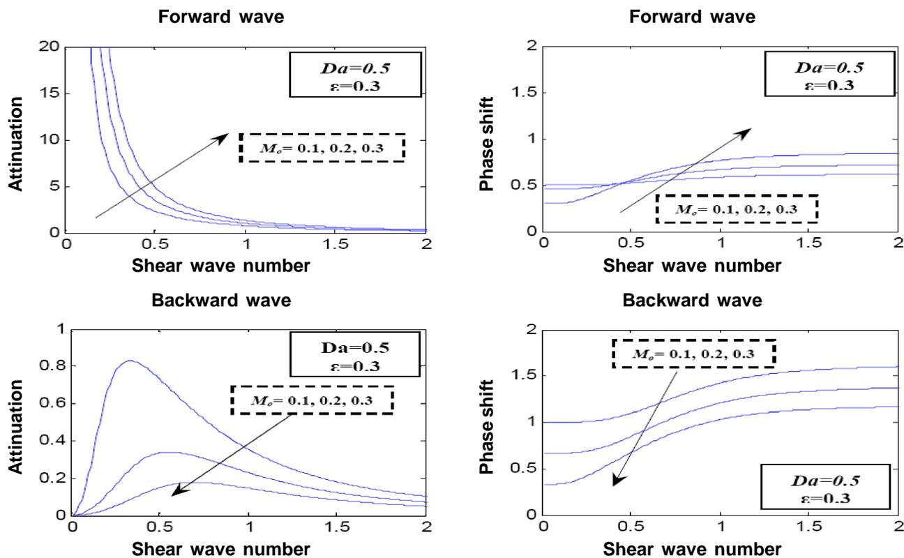
Figure 6 : Forward and backward waves attenuation and phase shift at Darcy number ( $Da=0.5$ ) and porosity ( $\epsilon=0.3$ ): (a) forward wave attenuation (b) forward wave phase shift (c) backward wave attenuation (d) backward wave phase shift
