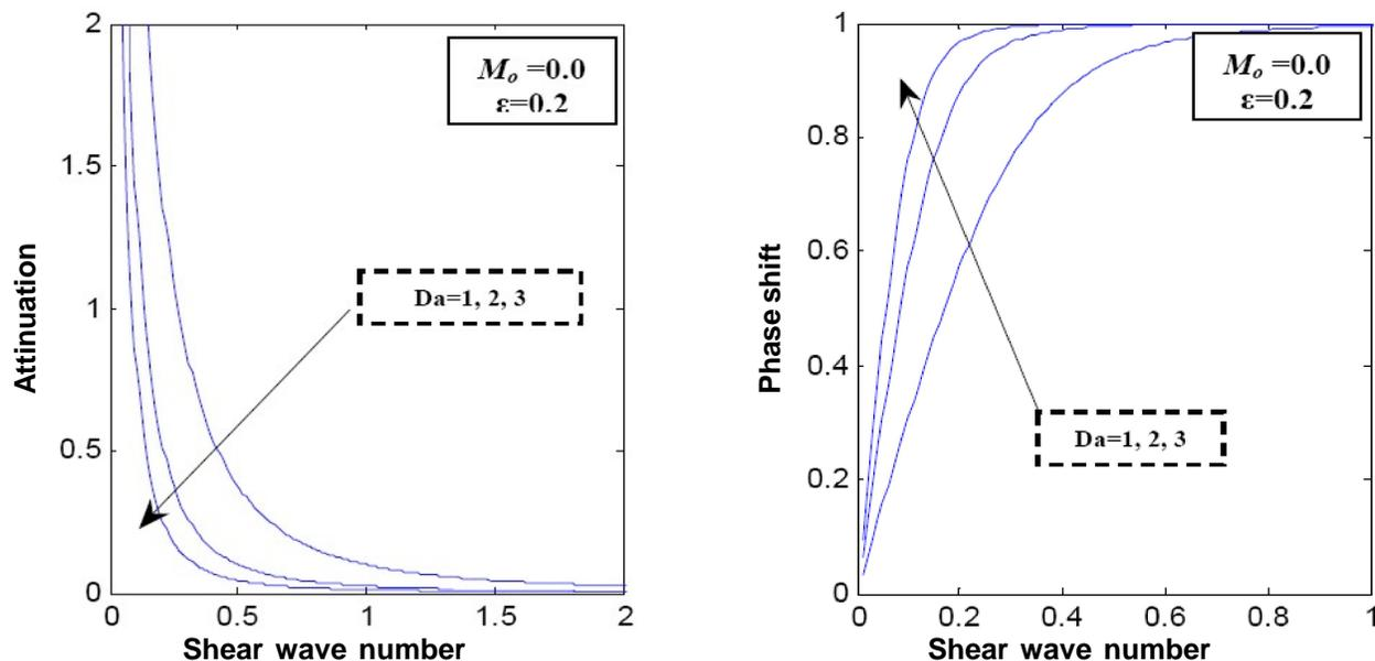
Figure 4 : Attenuation and phase shift of stationary ( $M_o=0$ ) fluid porosity ( $\varepsilon=0.2$ ) at various Darcy number ( $Da$ ): (a) attenuation (b) phase shift
