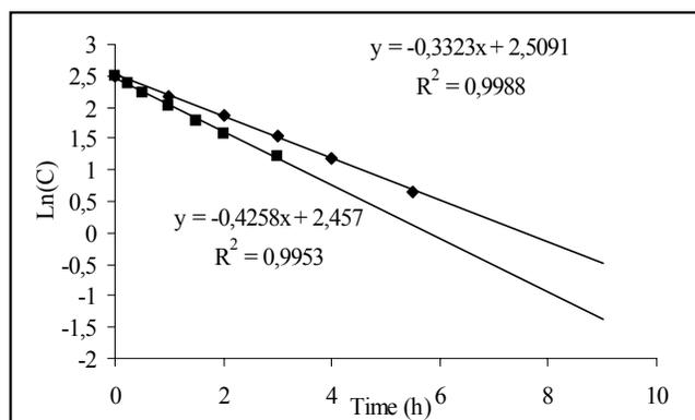
Figure 6: plot of Ln(C) versus irradiation time
