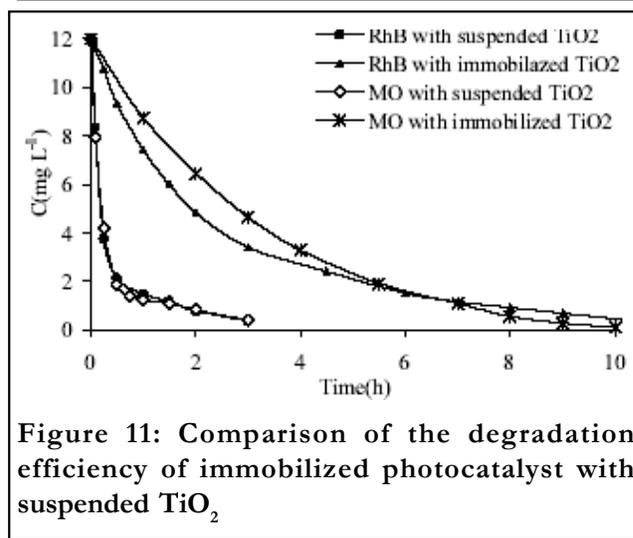
Figure 11: Comparison of the degradation efficiency of immobilized photocatalyst with suspended  $\text{TiO}_2$
