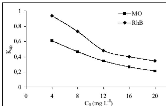
Figure 7: Variation of the apparent rate constant of degradation versus initial concentration of MO and RhB
