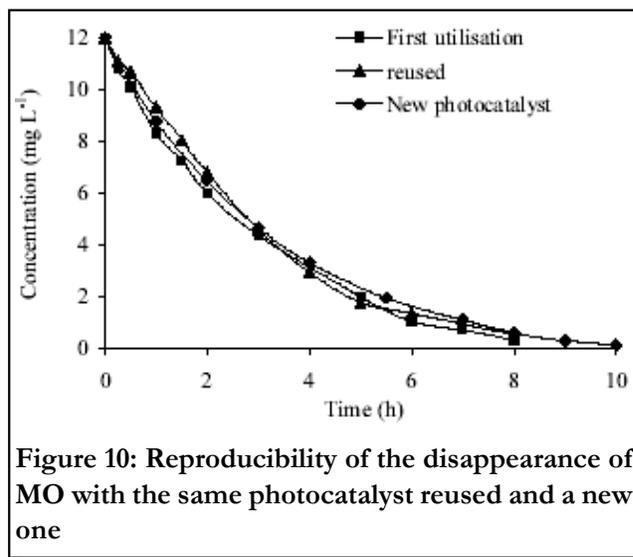
Figure 10: Reproducibility of the disappearance of MO with the same photocatalyst reused and a new one
