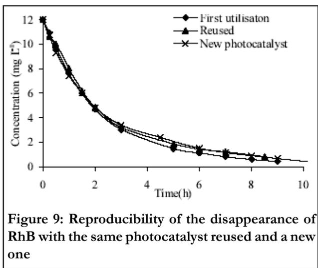
Figure 9: Reproducibility of the disappearance of RhB with the same photocatalyst reused and a new one
