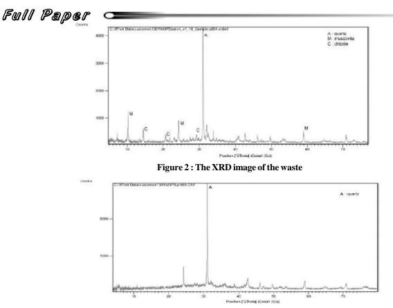
Figure 3 : The XRD image of the sintered single soil sample of W
