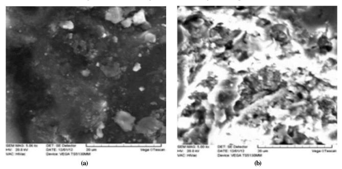
Figure 4 : The SEM images of a) the body made by the waste (100%W) and b) the parent ceramic body (40%A1, 18%A2, 22%B, 12%C1, 8%C2)
