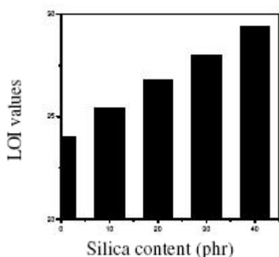
**Figure 3: Variation of limiting oxygen index value (LOI) of different concentration of silica filled DCSBR**
