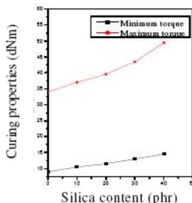
Figure 2: Maximum torque and minimum torque of different content of silica filled DCSBR
