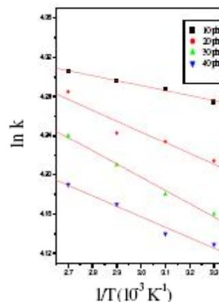
Figure 9: Arrhenius plots for the extraction of the unbound and loosely bound rubber of silica filled DCSBR compound
