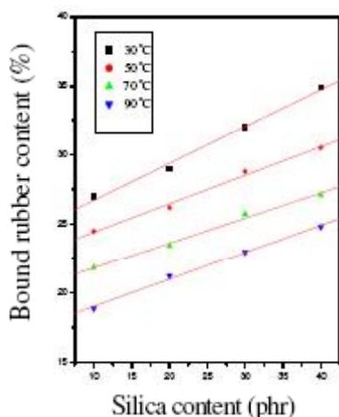
Figure 8: Variation of bound rubber content of silica filled DCSBR compound
