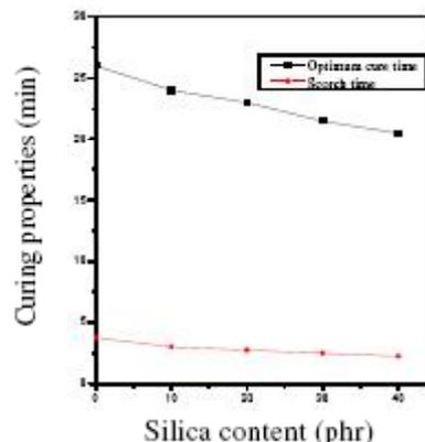
Figure 1: Optimum cure time and scorch time of different content of silica filled DCSBR
