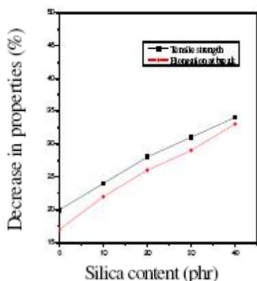
**Figure 5:** Decrease in percentage of tensile strength and elongation at break of silica filled DCSBR after aging at 72 hrs
