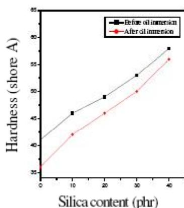
Figure 7: Change in hardness of silica filled DCSBR before and after oil immersion
